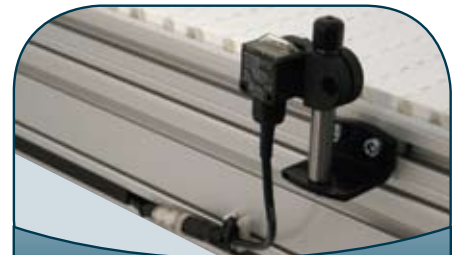
T-Slots and Quick Slots for Accessory Mounting
